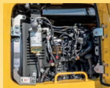
Centralised arrangement of filters
