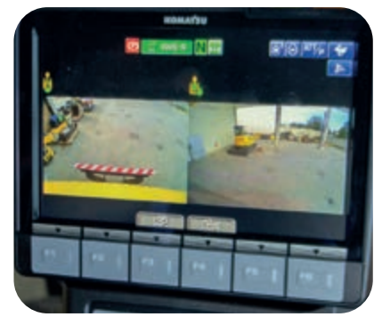
Rear- and side-view camera system
