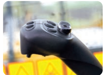
Convenient, ergonomic and precise control: joysticks with proportional control button for attachments
