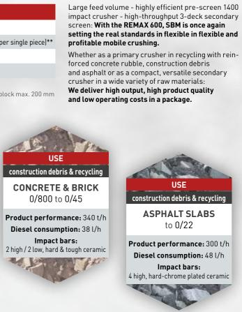
Easy one-piece transport - minimal set-up times -- optimal logistics on site
